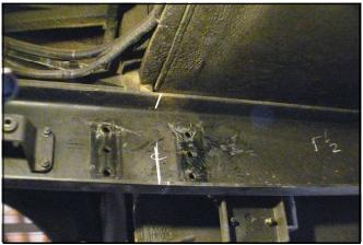
After properly blocking and lifting with safety supports in place, remove cross member and spring hangers. Mark center of spring hanger, as pictured, for placement of frame plates — left and right.
