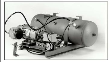
Air kit available with compressor, tank, regulator, pressure control and necessary valves to protect air supply. Gauge and recovery light mounted as pictured. Light can be remounted in cab so that driver knows when compressor is running and monitor recovery time. Compressor and control switches each protected with separate resettable fuses (push in to re-set).
