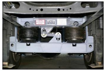
Superide installed on 4200 International chassis. Note the leveling jacks and adequate suspension clearance.
