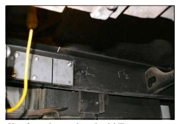
Place frame plates as pictured and drill necessary holes.
